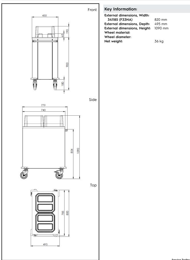
Service Trolleys Plate Dispenser Trolley, 2 cylinders - Ø180-300 mm
